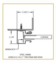
Universal mount 2" deep 16 gauge galvanized steel guides require no pre-installation modifications for steel or concrete and masonry block applications. Guides have deeper engagement, which allows the curtain to stay in place under more severe wind conditions.
